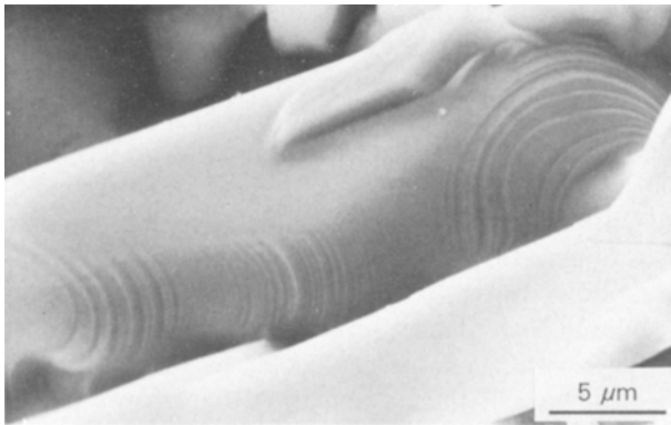
Figure 4 Scanning electron micrograph of the as-grown (010)/(100) surface of a different domain; step trains are shown.
