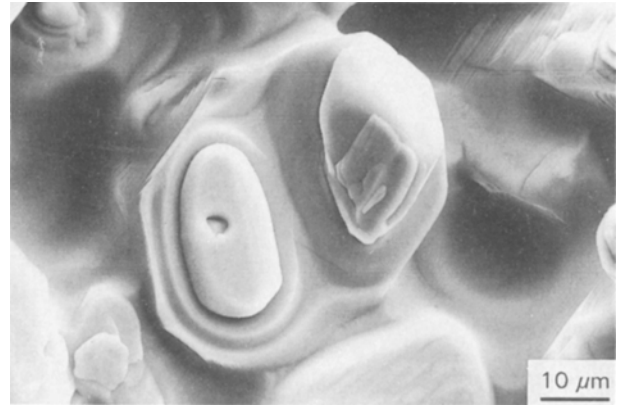
Figure 9 Scanning electron micrograph of an octagonal-shaped macrospiral distorted during the growth by the presence of two Y_2BaCuO_5 particles.
